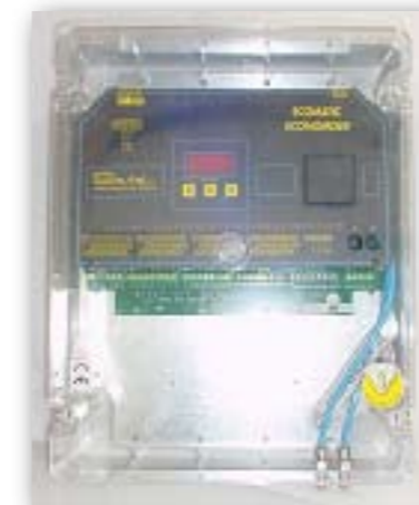
Differential pressure gauge with generator
